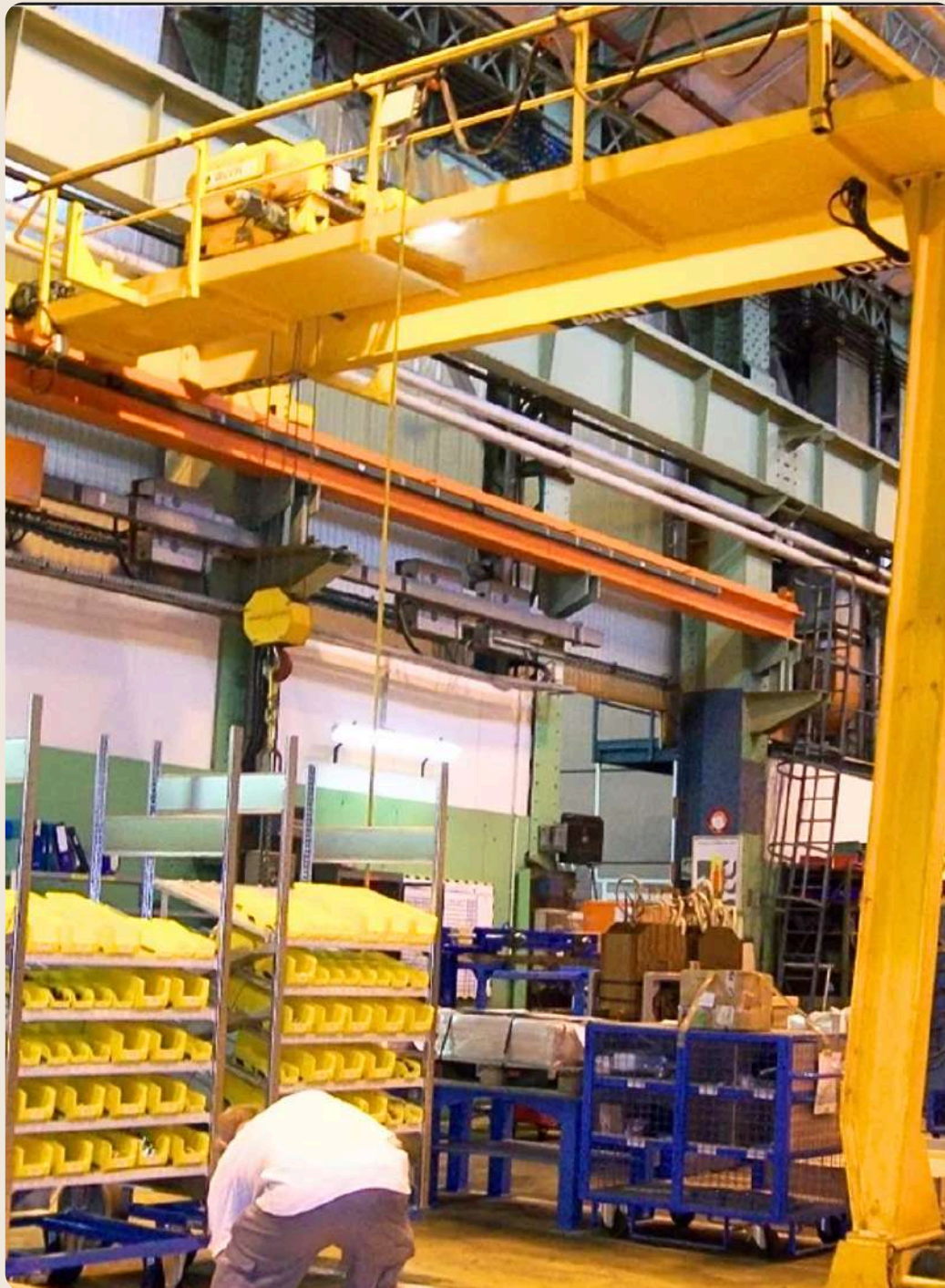
Semi Girder Gantry Range: 1000 kg to 100000kg
