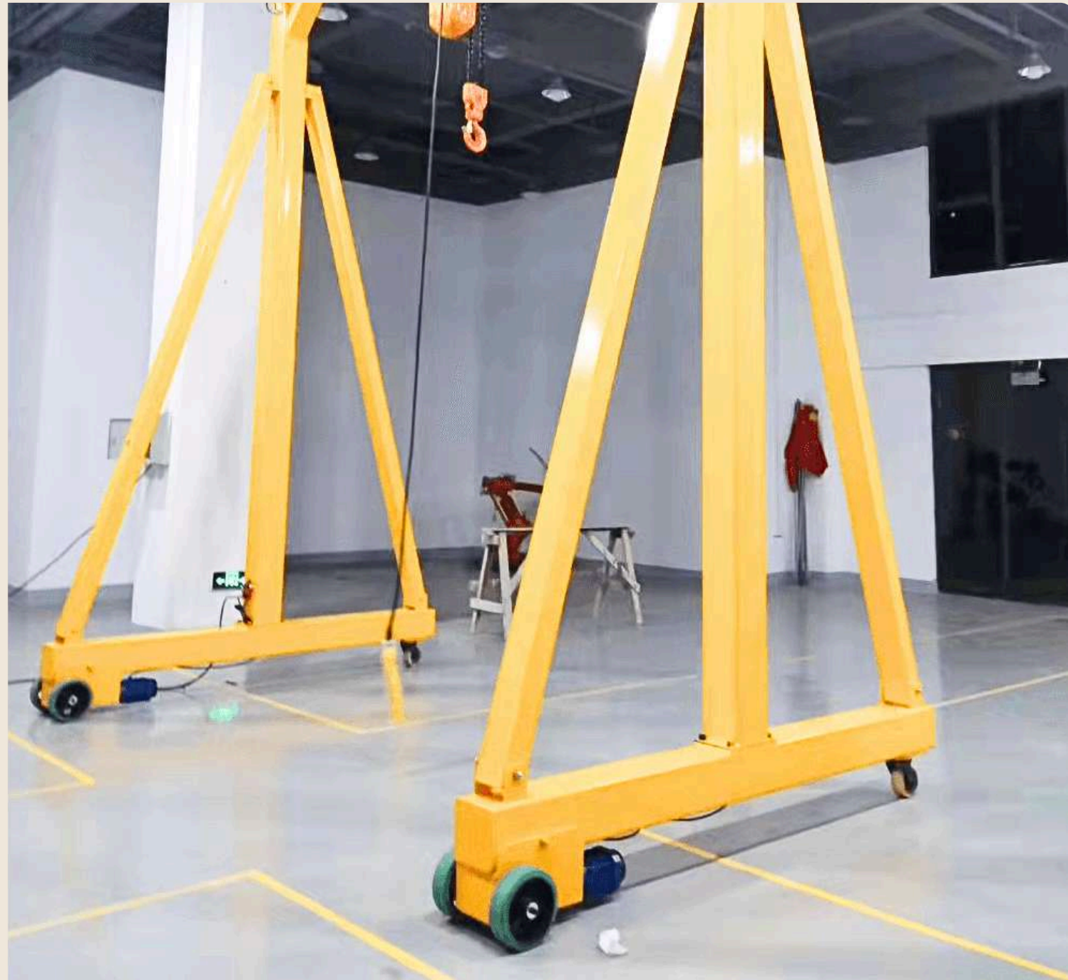
Portable Girder Gantry Range: 5000 kg to 5000kg
